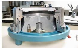
The mould components is designed to maximum cooling effect which consist of a graphite rings, an adapter plate, an adapter plate pressing, a connecting sleeve, a seal ring and a pressure equalization ring. There is a double-row cooling hole on the mould which enhances cooling effect and improve the quality of billets.
