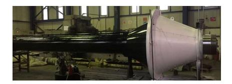
Type Single acting, internally guided 6800 mm Max Max stroke Cast 6500mm length Ø420mm Cylinder rod diameter Angular rotation 0,1 degree max
